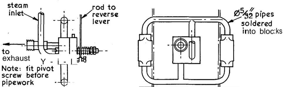
REVERSE 'VALVE & PIPEWORK
