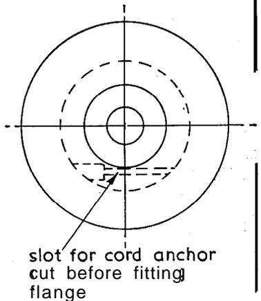
slot for cord anchor cut before fitting flange
