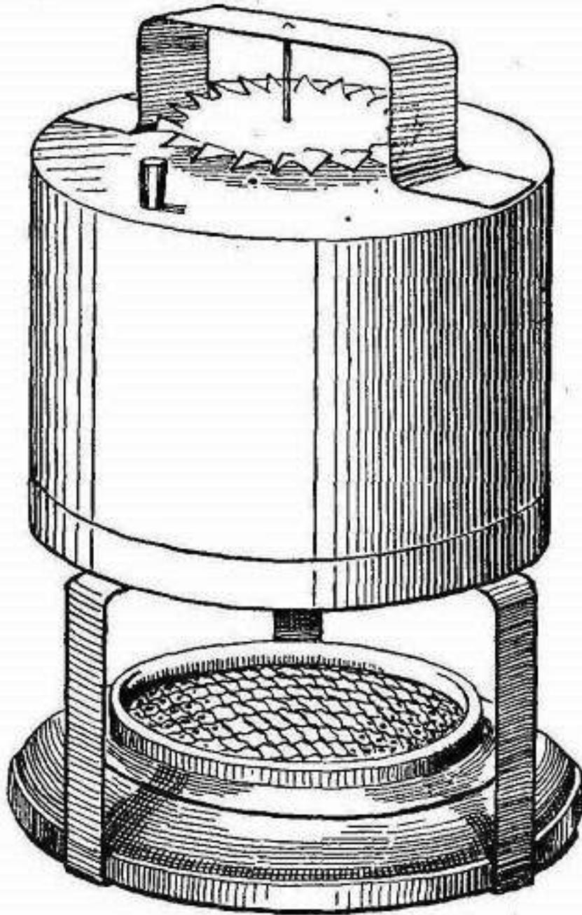
FIG. 67.—Simple steam turbine.
