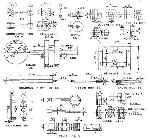
Although being primarily a high-speed boat engine, it would serve equally well as a stationary unit for dynamo driving, pumping, etc. For boat work it should give speeds up to 15 m.p.h. on
