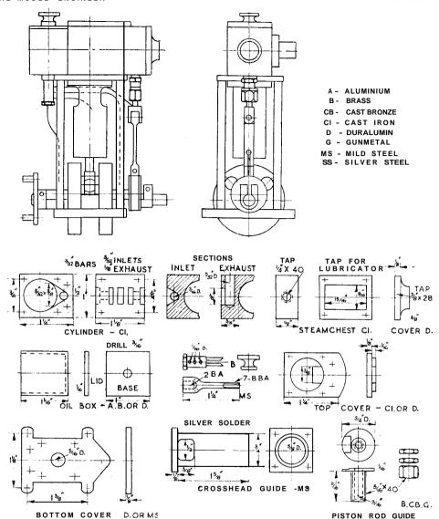
Start with the cylinder-block and see that you get a piece of good cast-iron. In my time, I have cut bits off flat-irons, garden gates, weights, etc.
