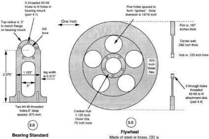
1/4 inch thick aluminum Height to bore center 2.375" Width at base 1.6875" Bore Dia .625" to fit bearing mount (part 4.1) 4.062 Inch
