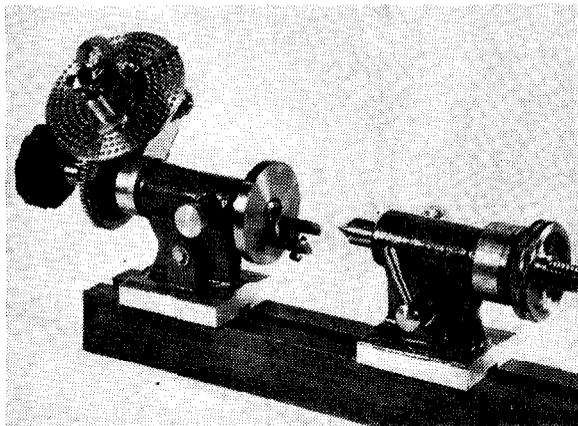
be used for finishing if it does not have to take out more than a few thou. At the same setting the back edge of the base, the shouldered end of the headstock, and the recess in the tailstock boss, can be machined. Mandrels, of the two appropriate sizes, may be used to mount the castings for facing off the front ends, and the front edge of the base, which should be flush.
