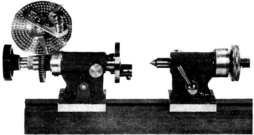
SOME form of indexing is a necessity in many milling operations, and though the rotary milling table already described can be adapted to indexing about a vertical axis, it is not suitable for dealing with work pieces of any substantial length. A horizontal indexing head has a much wider range of application and can be used in gearcutting, fluting taps, reamers and other cutters, and making long splines or keyways, all of which are commonly encountered in light engineering practice.
