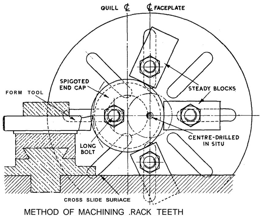
always caused by the incorrect adjustment of the steady pads, so that the work is forced out of true centre alignment. If the back centre is used to support the end of the bar while the radial position of the pads is adjusted and locked, no trouble should be encountered.
