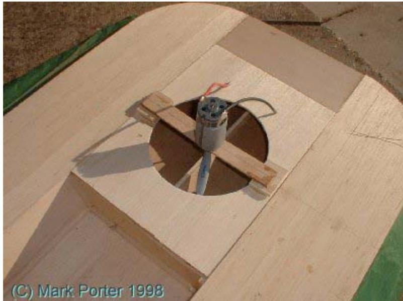
The inner wall of the lift duct is made from a sheet of 0.4mm plywood, with the grain of the outer faces running along the longer dimension. Gently roll the duct wall and fit in place. Mark the overlap and remove the duct wall. Glue the duct joint along the overlap line. When the glue is dry, fit in place and then fix with glue.
