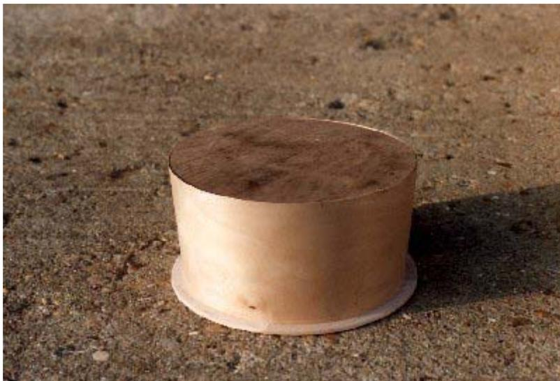
Take the plywood disc which was removed when the duct ring was cut out and fit this inside the duct inner wall, in the end opposite the duct ring. This should not be glued, but is just to keep this end of the duct circular while the outer wall is fitted. Glue the outer wall to the duct assembly. When the glue has dried, remove the disc and trim and sand the duct ends.
