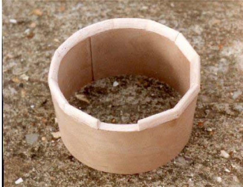
Cut the 24 leading edge sections from balsa strip to match the sections marked on the face of the duct ring. Balsa strip is available already formed into a leading edge section. If you cannot obtain this, use 12.5mm (1/2") square strip. Glue the 24 sections to the face of the duct ring. Allow the glue to dry and sand to form a smooth, rounded lip.
